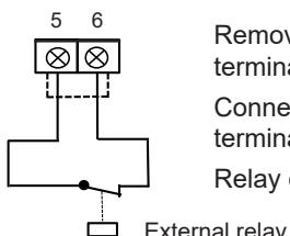
Remove the existing cable between terminals 5 and 6.
